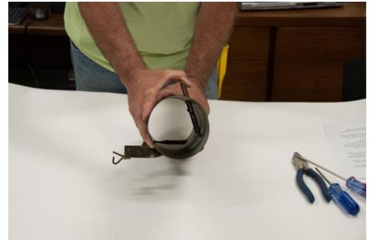
To fix a bend, put a broom handle or similar size bar through the trap on the dog and safety side, between the strike bar and inside of the tube trap. Lightly push the top of the strike bar toward the broom handle you have inserted into the tube trap, pushing lightly until the strike bar has been straightened.
