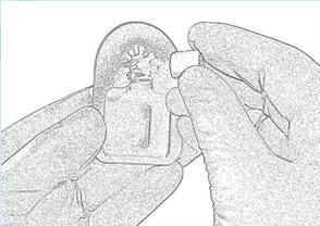
**Step 1:** Push the tablet gently but firmly into the holder, leaving approximately 50% of the tablet exposed.
