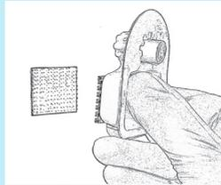
**Step 2:** Remove plastic protection from the sticky mounting on the back of the holder.
