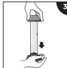
**3** Replace tube. Hold by protective cap and press down firmly onto base.
