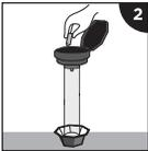
**2** Open the base and install 3 AA batteries.\*
