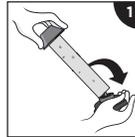
**1** Remove used tube from base. Hold from the cap and pry off from the base. Dispose used glue tube.
