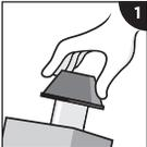
**1** Slowly lift the GLOstik™ by holding the black protective cap. The orange cap indicates the replacement glue tube (for later use).
